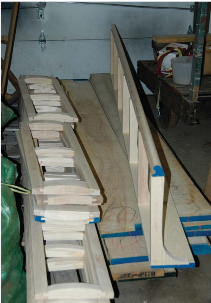
Cleveland Center Entrance Trailer 2365: The second center entrance car receiving work in the shop is the beautiful Cleveland trailer acquired from the Lake Shore Electric museum collection. One of the few remaining tasks to complete the car is fabricating the seats. Here seat frames, identical to those made for motor car 1227, are taking shape and soon will have springs, padding, and rattan covering added.
