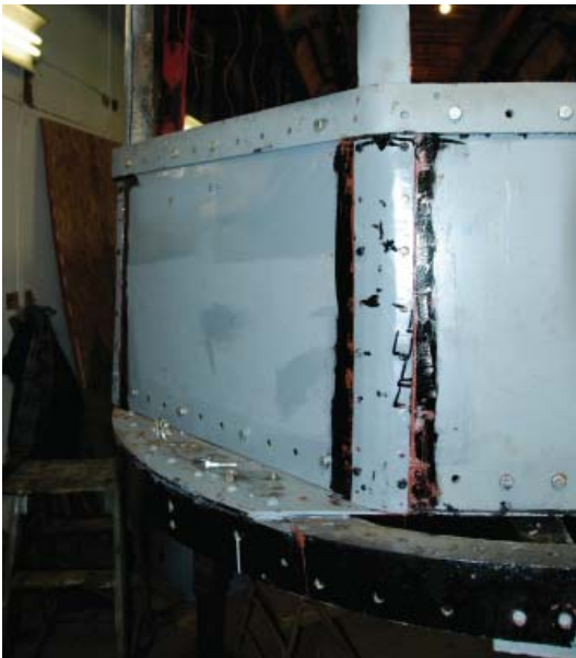
Boston Center Entrance Car 6131: The final pieces of new sheet metal are being aligned and prepared for riveting (left above) and corroded underfloor structural frame members are being built up with welding. Meanwhile, the complicated control switch group (above right) for the car's ABPC 32 multiple unit control has been overhauled and installed below the floor near the center doors.
